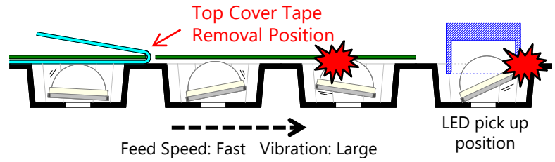
Figure 5. Examples of Correct/Incorrect Top Cover Tape Removal Positions
